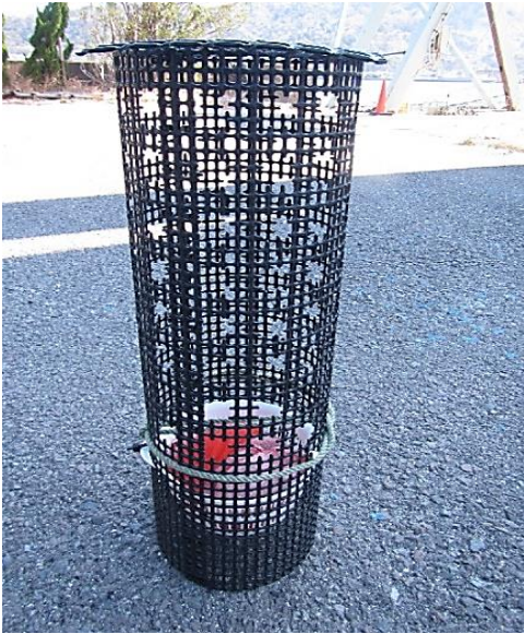
Fig.7 A container for transplanting S.horneri thallus to be placed on the artificial seaweed reefs. A round white plastic basket containing a 1kg sandbag was inserted into a cylindrical shape made of trical net and fixed in place.
